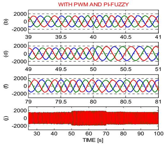
**Fig. 8:** Rotor current of DFIG (i, j); Rotor current during transient state (a, b)
