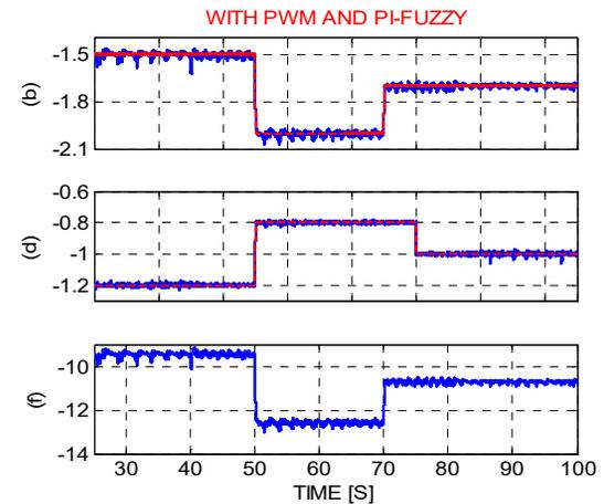
**Fig. 9:** Active (a, b), reactive (c, d) and torque (e, f) output power of DFIG
