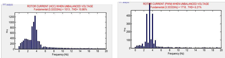
**Fig. 12:** THD's rotor current when unbalance voltage
