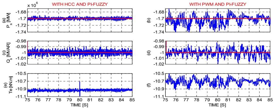
**Fig. 10:** Active (a, b), reactive (c, d) and torque (e, f) power during unbalanced voltage (balanced again from the 80th second)
