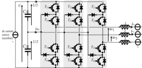
Fig. 5: Three-phase three-level VSI
