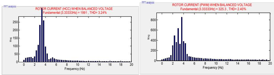
**Fig. 13: THD’s rotor current when balance voltage**
