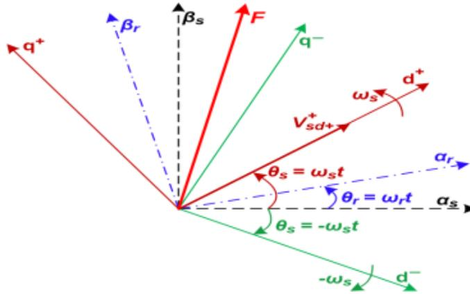
**Fig. 1: Relationships between  $(\alpha,\beta)_s$ ,  $(\alpha,\beta)_r$ ,  $dq^+$  and  $dq^-$  reference frames**
