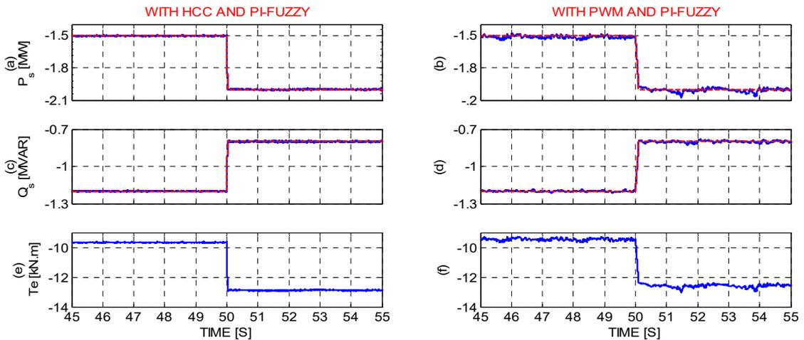
**Fig. 11:** Active (a, b), reactive (c, d) and torque (e, f) power during transient state
