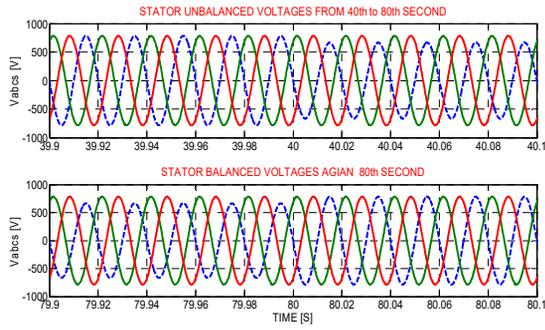
**Fig. 6:** The grid voltages are unbalanced from the 40<sup>th</sup> to 80<sup>th</sup> second
