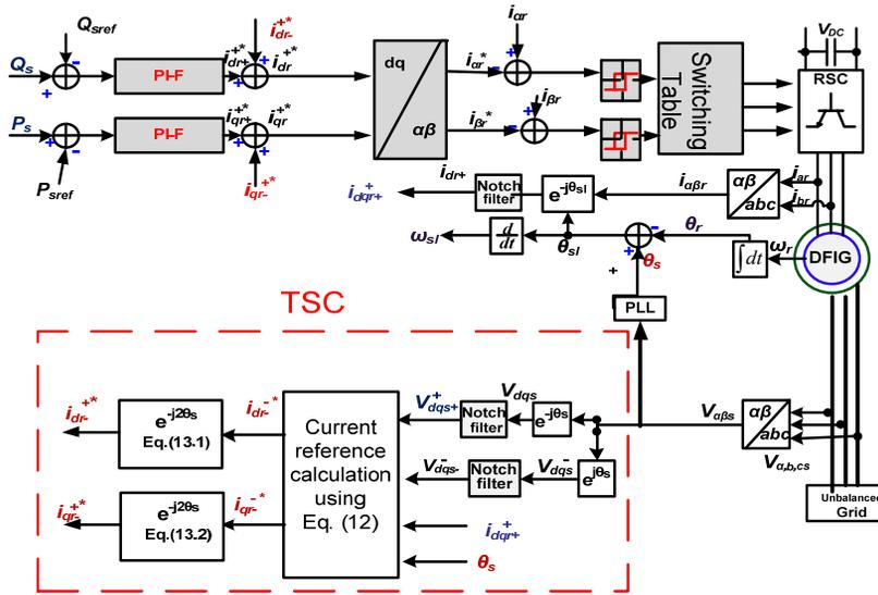
Fig. 3: Proposed control structure with HCC, TSC and PI-F
